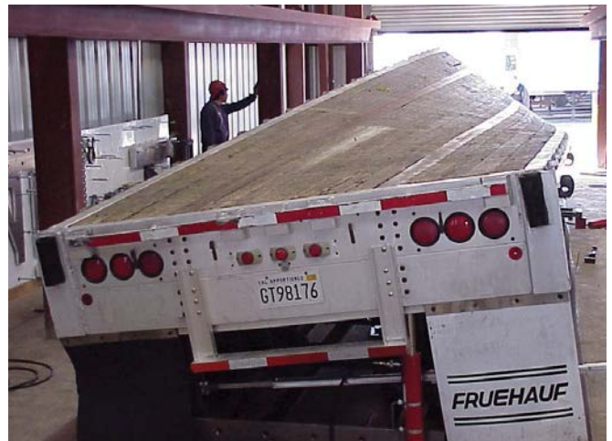
This twisted trailer is being corrected with Trailer Twisting Tools. Floor "I" Beam setup works primarily with trailer corrections.
