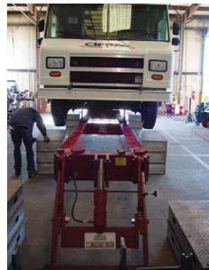
Portable Aluminum Ramps allow even the lowest profile vehicles enough clearance to traverse the Bee Line Drive Over Frame Press.
