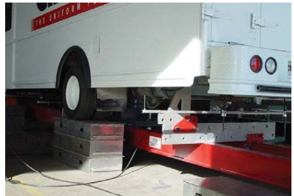
Portable Aluminum Ramps allow even the lowest profile vehicles enough clearance to traverse the Bee Line Drive Over Frame Press.
